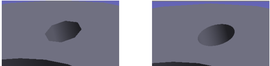
Figure 5-21. Max trimmed edge angle: 65 (left) and 15 (right).
