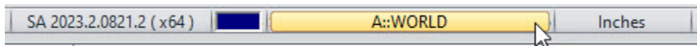
Figure 9-2. The Working frame selection control at the bottom of the SA graphics window.
