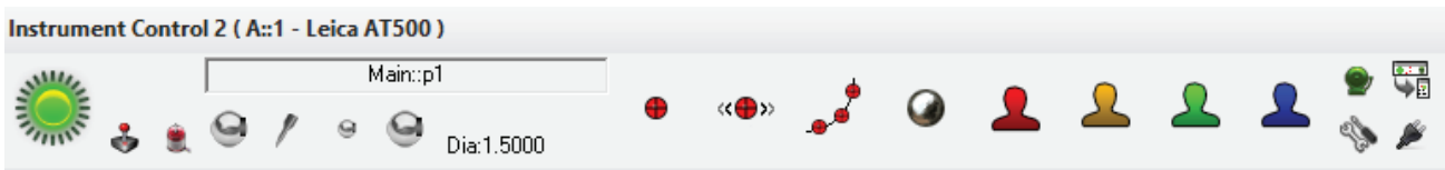
Figure 3-74. Instrument Control Toolbar is a simplified tracker interface to expand graphic space.
