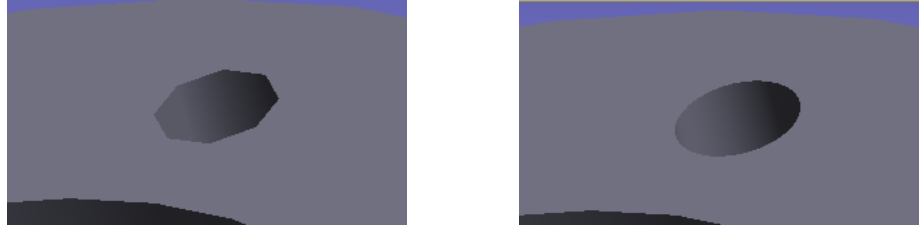
Figure 5-21. Max trimmed edge angle: 65 (left) and 15 (right).
