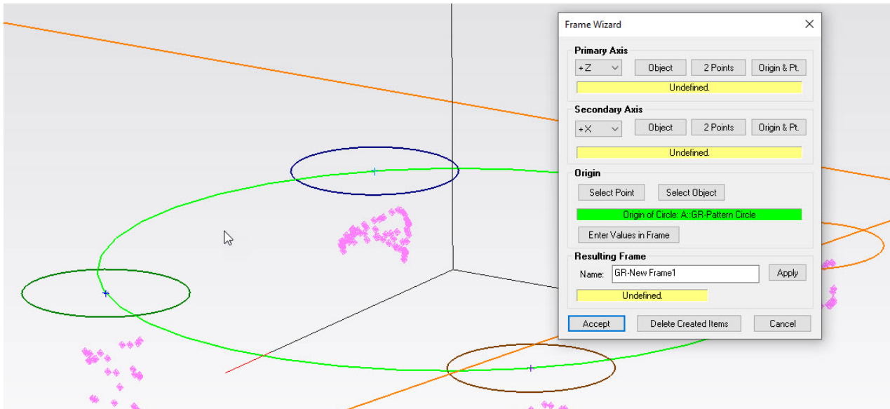
Figure 25-45. Selecting center circle as the reference for the new frame.
