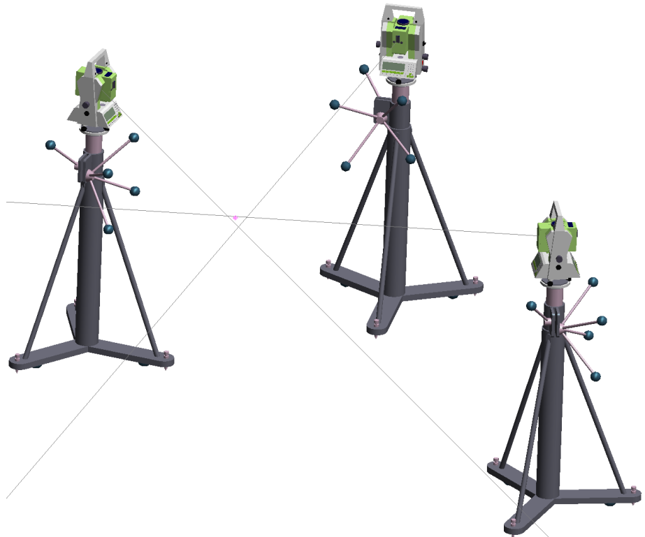
Figure 8-10. A measured target as computed by observations from three instruments (exaggerated for clarity).
