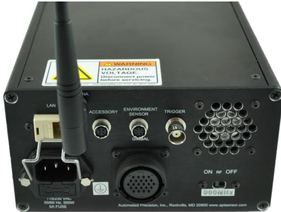
Figure 2: API Tracker3™ wireless configuration
