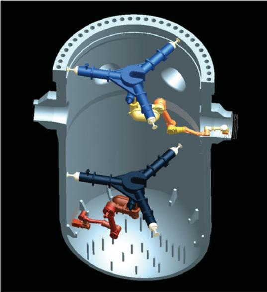
The full dexterity of the robotic arm is used to deliver transducers to inspect the nozzle inner radius and the nozzle bores including the deeper pipe-to-safe-end and bi-metallic welds. A unique base configuration allows the arm to “flip” either above or below the base to support different examination configurations. The entire weight of the system in water is approximately 100 pounds (50Kg).
