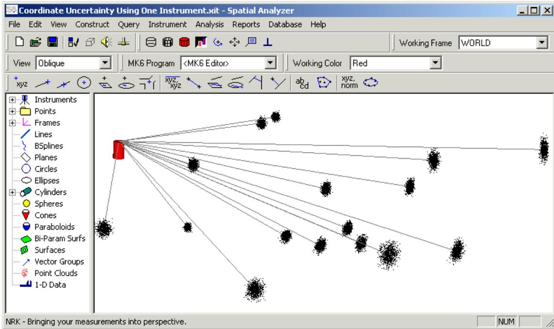
Figure 3.4: Uncertainty Clouds (Gaussian) for Bundle Test Points
