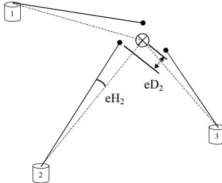
Figure 2.1: Bundle Residual Components
