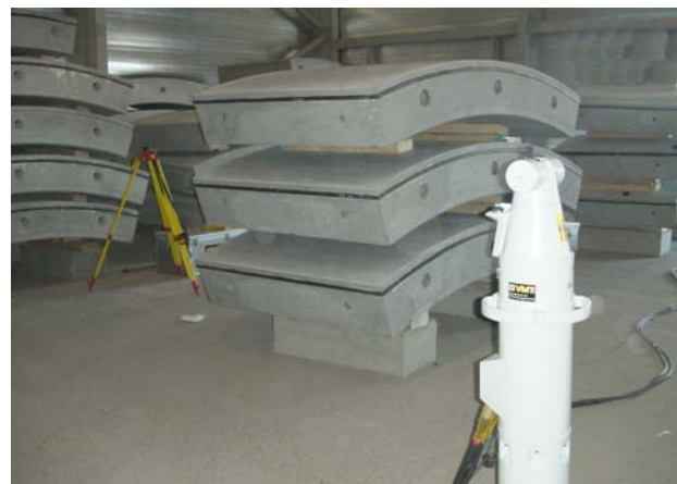
Figure 5 Stacked segments for rapid measurement
