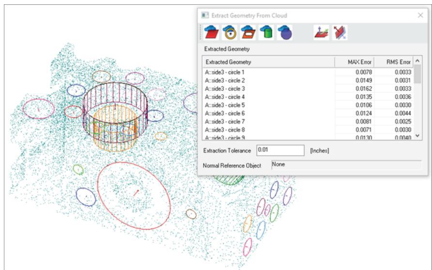
A second surface circle extraction option has also been added that allows a user to detect geometry within a specified proximity to a set of nominals and build the fit geometry from point clouds where only the surface can be scanned (such as is the case when working with sheet metal). This function does not require CAD, but can use a set of reference geometry directly as guidance.
